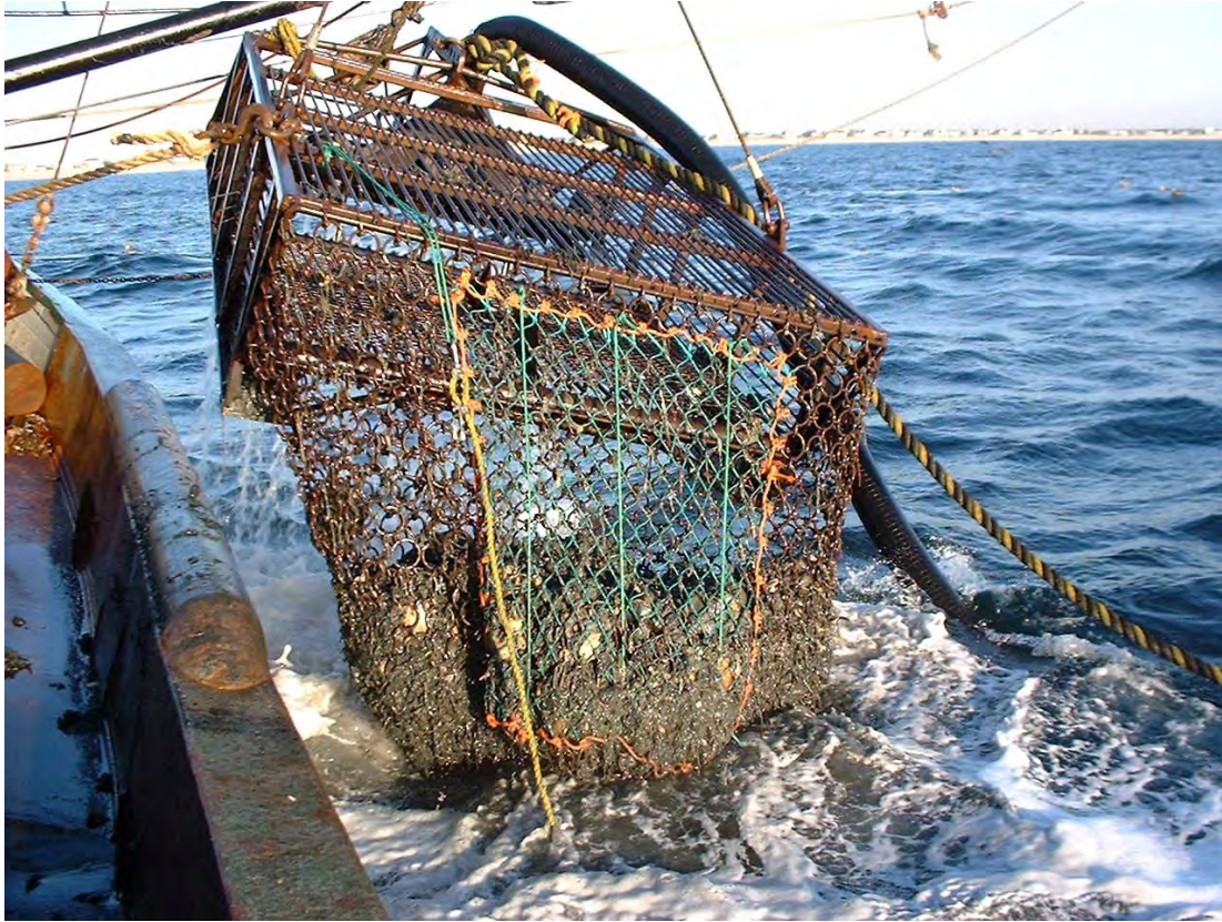
Appendix A1, Figure 4. The inshore commercial clam dredge used for the New York surveys. Photo courtesy of Jeff Normant, NJDEP; William Burton, Versar, Inc.; and Beth Brandreth, USACE.
